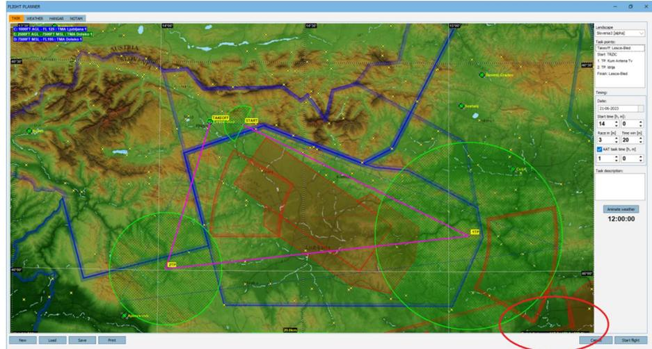
To plan your route you can drag the magenta lines in the AAT sectors by holding down shift and moving the turnpoints with the mouse. In the bottom right of the map you will see the task distance changing. To help you plan, there are dotted blue and red lines. The blue lines will give you the maximum possible distance, and the red lines minimum distance. If possible, choosing a route that avoids airspace and mountains will in general give you the fastest possible speed.
